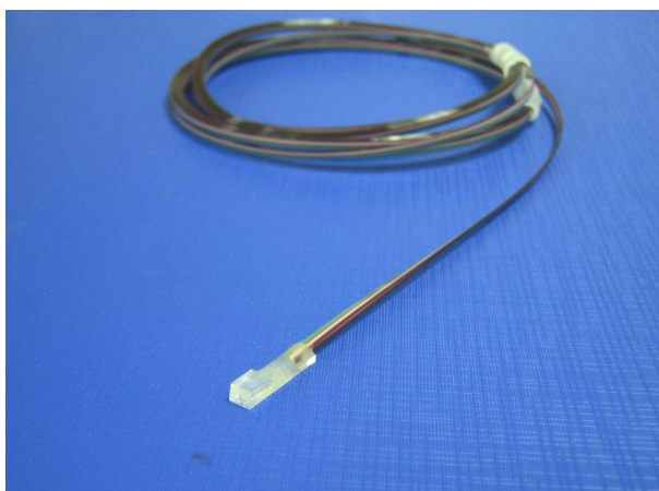
Fig. 3. Appearance of the bonded fiber array packages.
